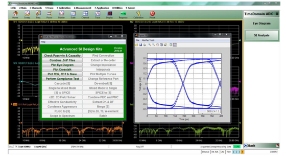
MS46500B series advanced time domain Option measurement showing signal integrity and eye diagram tools
